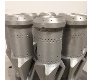
Additive manufacturing for R&D speed when developing next generation of green burners
